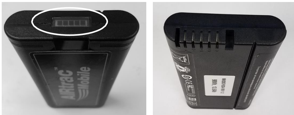
Figure 12: Battery Charge Indicator Showing Full Charge and Battery Terminals
