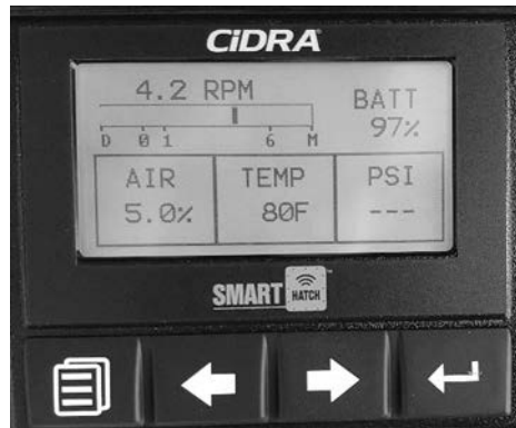
Figure 25: In-Cab Display (Measuring)
