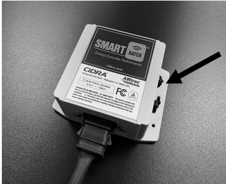
Figure 23: Receiver Module Pairing Button and LED
