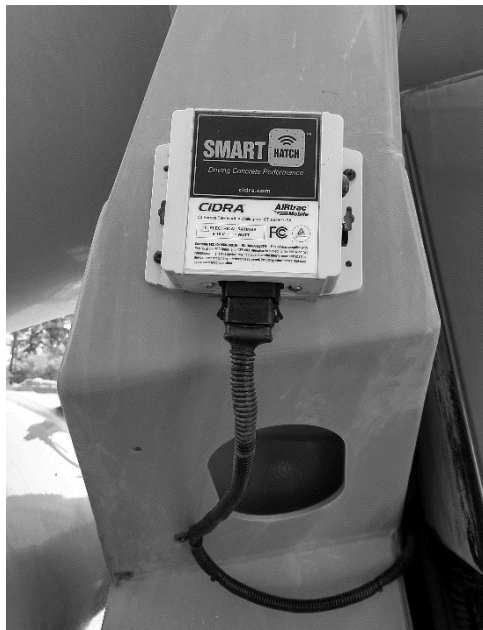
Figure 13: Receiver Module Mounted to Back of Truck Cab
